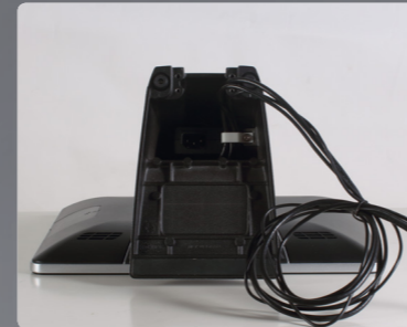
The adaptor is hidden inside the top of the stand
